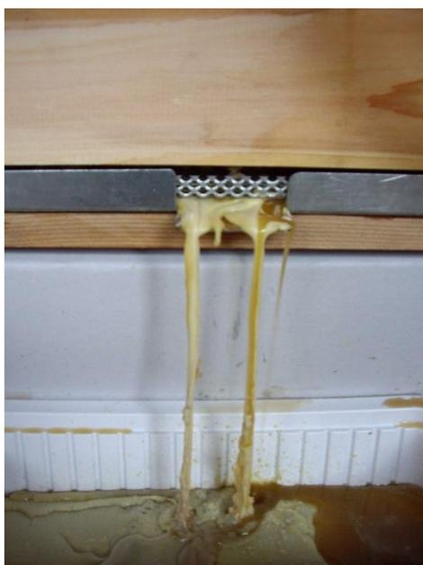
**Figure 7, hot wax collecting from a steam wax extractor.**
